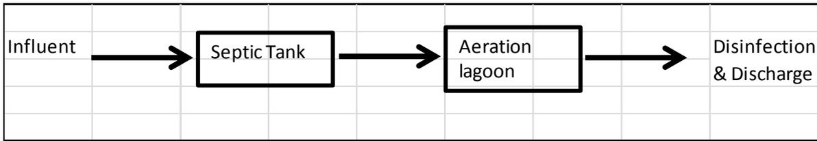
**Figure 2: Basic aerated lagoon treatment flow diagram**
