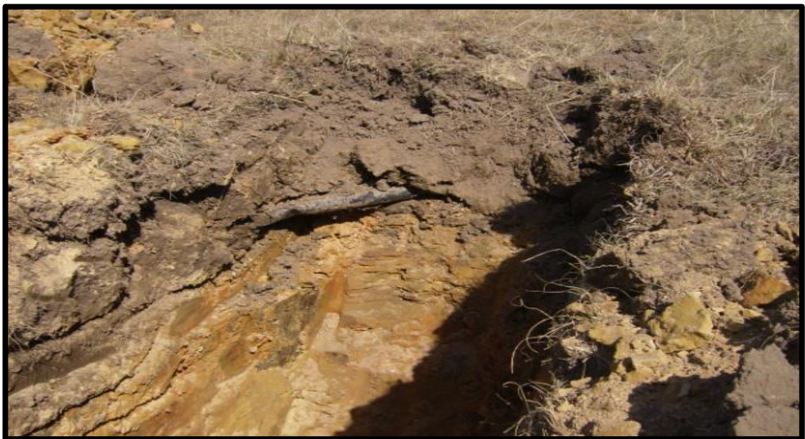
FIGURE 4-2: COLLUVIAL SOILS UNDERLAIN WITH BEDROCK
